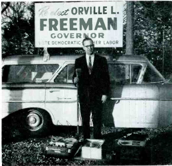
Sound truck used by Minnesota's incumbent Governor Orville L. Freeman employs a 60 watt Bogen mobile public address system amplifier, a Viking cartridge tape deck, and a Bell & Howell conventional tape recorder.
