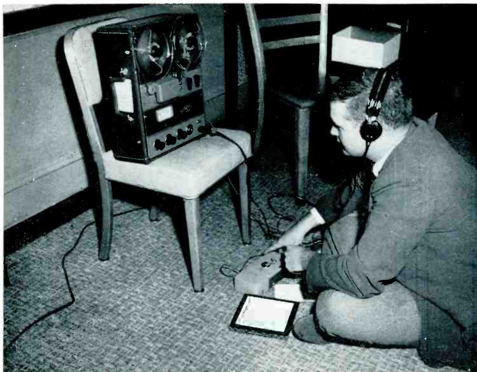
Miniature battery operated tape units are often used for on-the-spot campaign recording, then dubbed onto conventional tape reels for subsequent use. A Mohawk Midgetape is being used here feeding to an Ampex 600.
